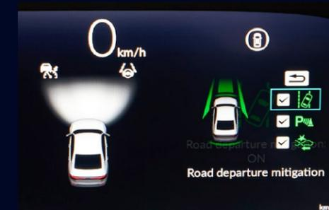
The Honda SENSING™ features can be fully customized in the TFT meter.
