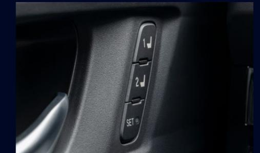
Accord comes equipped with an 8-Way Power seat height adjustment for the Driver's seat, and 4-way seat height adjustment for the passenger. Memory seats are a great addition that can be set to the individual remote key fobs, so you never have to adjust your seat again.
